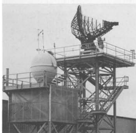
SPS-49 air search radar at the Sperry Land Test Site for the Perry class combat system. The radome is a Mk 92 system. Sperry
