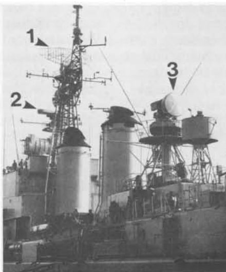
DRBV-22A (1), DRBV-50 (2) and DRBC-32 (3) radars as fitted to D'Estrées, 1979. STEFANO CIOGLIA
