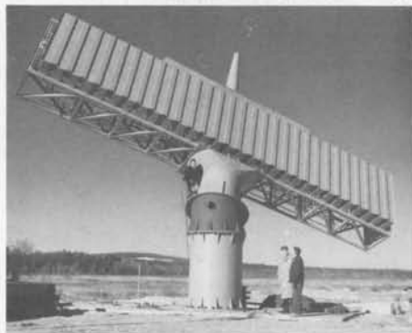
SPS-38 anti-ECM long-range air search radar, showing stabilization.
