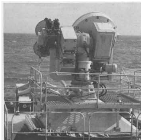
Type 910 Seawolf tracker, aboard HMS Penelope, October 1976. Note television tracker at left. MoD(N)
