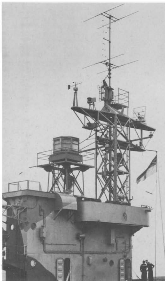
The British escort carrier Attacker, completing at Mare Island, shows standard British air search radars: the four dipoles of Type 279B on her mast, with the wires between clearly visible through their spreaders, and Type 272, the centimetric surface search radar, in its 'lantern.' The mast also carries the lightweight US aircraft beacon, YG.
