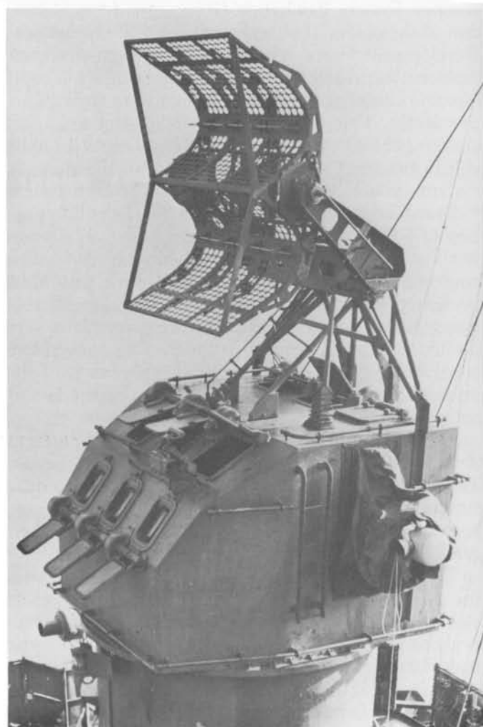
The Mk 4 (or FD) dual-purpose fire control radar epitomized the lobing technique; here one is seen aboard the destroyer Nicholas, January 1944. Upper and lower parts of the antenna produced two separate beams, slightly different in angle; the strength of the return from each could be compared, and the radar pointed at its target when they were equal. The related Mk 3 surface gunnery set employed a similar technique, in which the two halves of the antenna, split either vertically or horizontally (depending upon the version) produced alternative beams. In many later systems, the entire antenna switched rapidly between alternative beams so as to generate an error signal when it was off-target.
