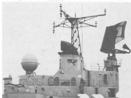
LW-02 radar antenna (right) aboard HMAS Vendetta, April 1977. The radome at left houses M22 fire control radar. GIORGIO ARRA
