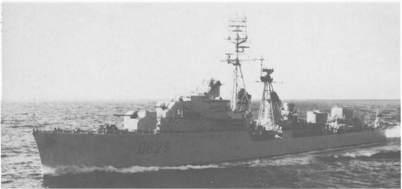
The French destroyer Cassard displays most of the early generation of postwar French naval radars in this July 1960 photograph. She carries DRBV-20 on her foremast, and the two-beam target indication radar DRBV-11 on her lattice mainmast. The antenna just below the big mattress of DRBV-20 is the associated IFF, presumably for a Mk X system, and below that (and forward of it) is the DRBV-30 surface search radar.
