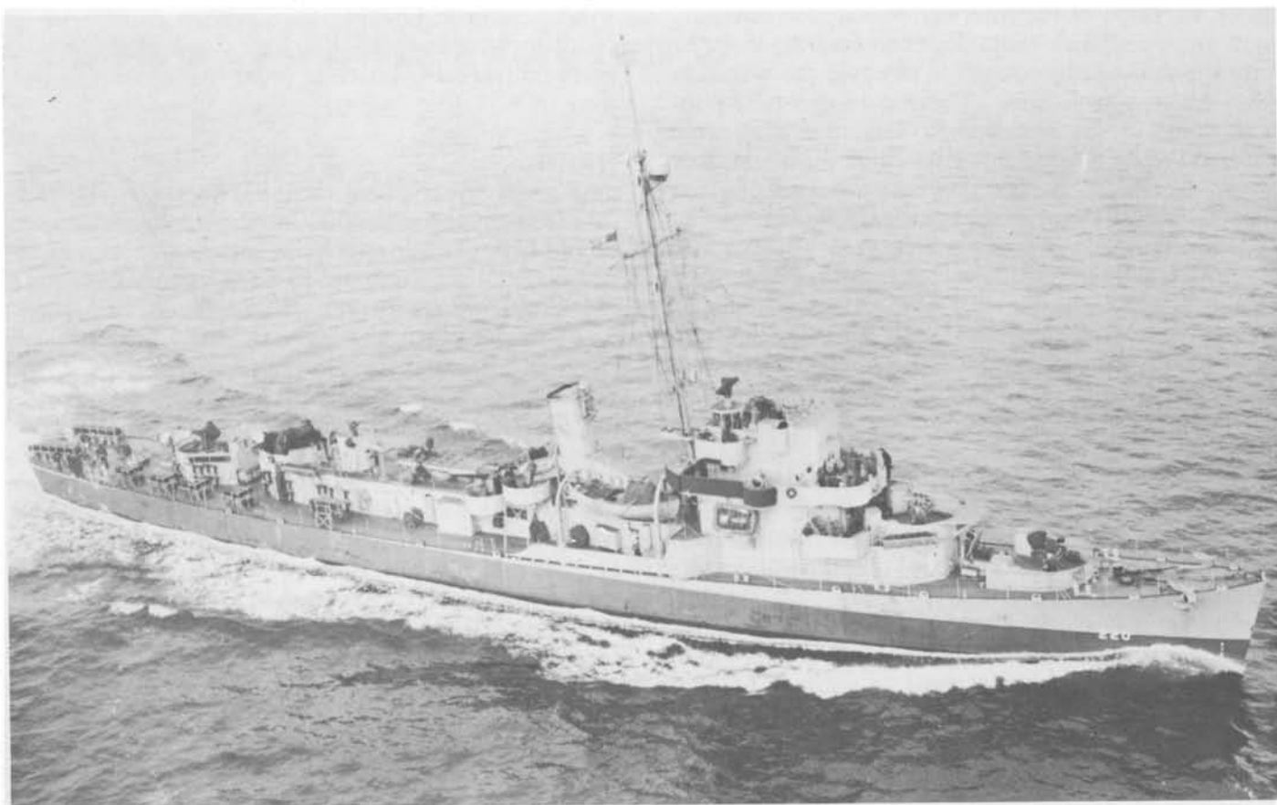
HF/DF was so important in the Battle of the Atlantic that many US escorts were completed with it in place of their air search radars. This is Francis M Robinson; she has an SL surface search radar. Later most such escorts received a short mainmast for their HF/DFs.
