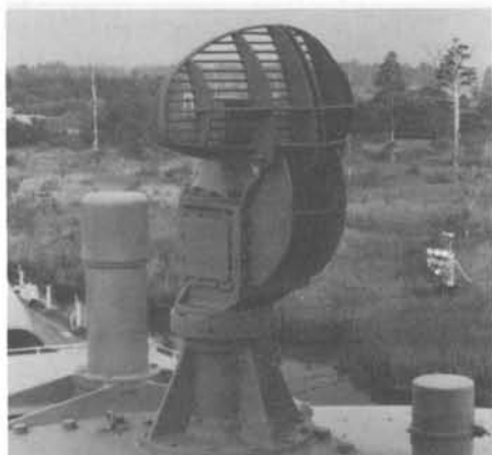
Mk 27 fire control radar on conning tower of USS North Carolina (memorial). This is the same antenna as SJ. A D BAKER III
