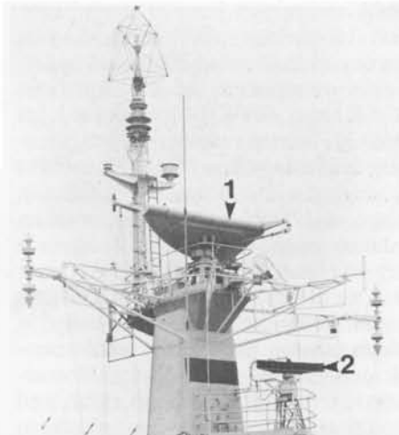
Type 994 (1) and 978 (2) radars, HMS Hermione, 1976. C & S TAYLOR
