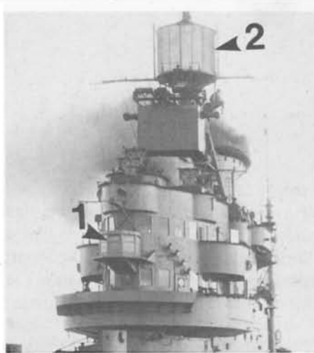
Type 271 surface search radar 'lantern' (1) and Type 72 aircraft homing beacon (2) aboard Indomitable, 1943. CONWAY PICTURE LIBRARY
