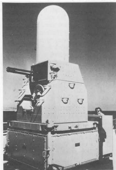
Phalanx (Close-In Weapon System). The two antennas are in the radome over the gun.
