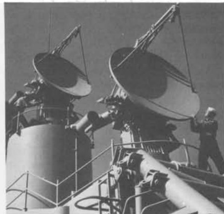
SPG-51 Tartar tracker-illuminator, showing feed details. BY COURTESY OF NORMAN POLMAR
