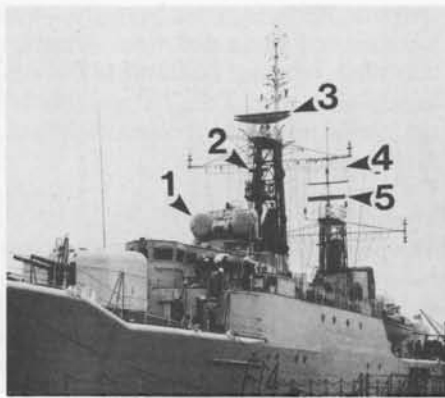
The frigate Leopard (30 September 1958) showing Types 275 (1), 974 (2), 293Q short-range air search/target indicator (3) and 960 long-range air search (4) radars, and IFF Mk X for the Type 960 (5).
