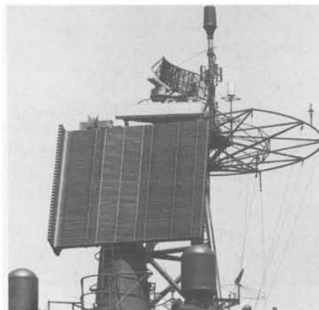
SPS-48. Note ground plane to separate the antenna from SPS-10 above.
