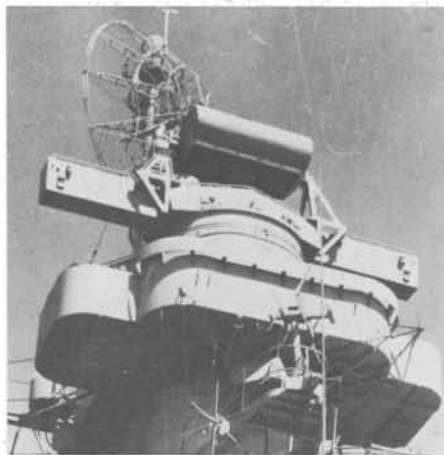
Mk 13 surface fire control radar, USS Iowa (July 1947), with SK-2 air search radar visible above and a TDY jammer below.
