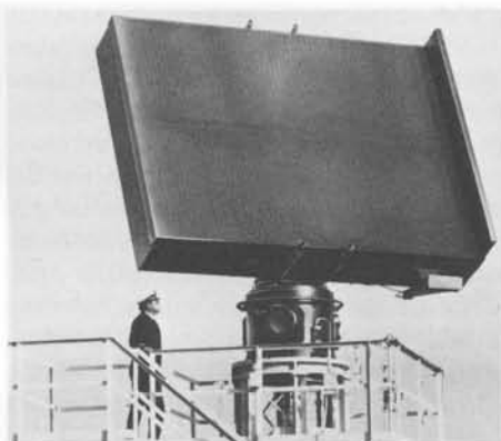
SPS-52C on test, showing the current planar array antenna, which differs considerably from earlier models.
