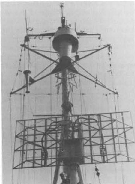
FuMO 21 with 4 × 2m mattress, DD-935 (ex-torpedoboot T35) 1945. Four fixed Sumatra search receiver dipoles are sited above. BY COURTESY OF ROBERT F SUMRALL
