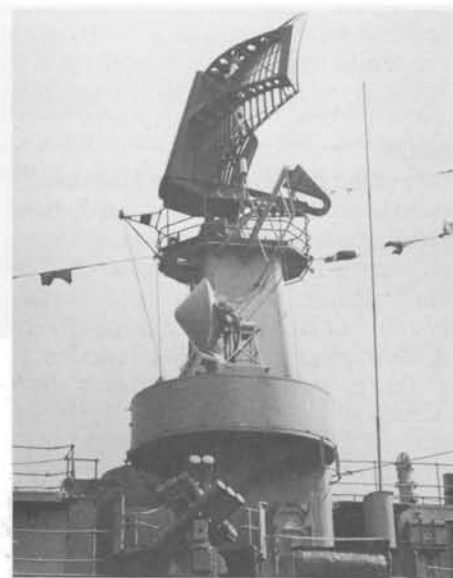
Evertsen in May 1978 showing an LW-03 antenna with M44 Seacat fire control radar below. Note chaff launcher at base of radar tower. PAUL BEAVER
