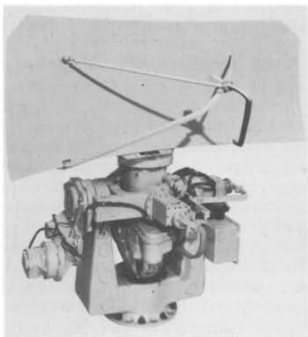
SPQ-9, with radome removed.
