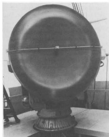
Mark 92 STIR (Separate Tracking and Illuminating Radar). SPERRY
