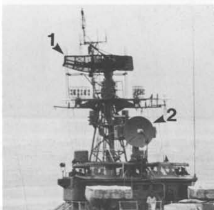
'Slim Net' (1) and 'Hawk Screech' (2) radars aboard a 'Petya' class patrol craft.
