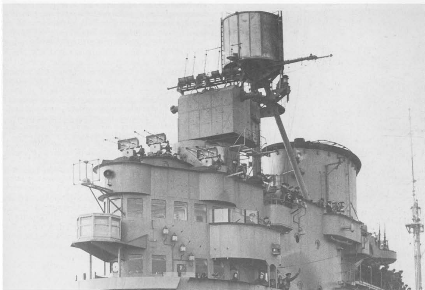
The carrier Indomitable (1943) shows several British radars characteristic of the early war period, particularly, on the bridge front, the 'lantern' of Type 271; above it is a medium-frequency radio direction-finder. The tripod mast is surmounted by the 'dustbin' of the Type 72 aircraft homing beacon, the British
