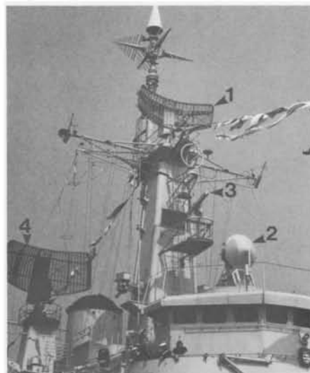
DA-04 (1), M45 4.5in fire control (2), Kelvin-Hughes Type 925 (3) and LW-03 (4) radars aboard Evertsen, May 1978.
