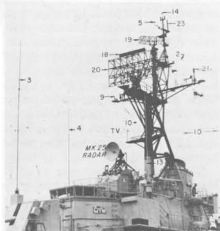
Foremast of USS Mansfield (DD-728), showing SPS-29 long-range air search radar (20) with IFF (18), SPS-10 (19) and Mk 25, March 1965.
