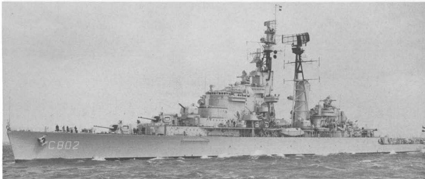
The cruiser De Zeven Provinciën illustrates most of the initial Dutch postwar naval radars. Fore and aft, she has an M45 director for her 57mm battery; a ZW-01/SGR-103 surface search radar; an M25 director for her 15cm main battery; a VI-01/SGR-104 height-finder; and a DA-02/SGR-105 target indication radar. The large tripod mainmast carries at its head an LW-01/SGR-114/06 S-band air search set.
