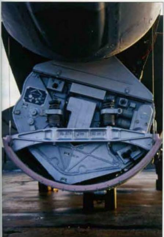
Top left: The underside of a MiG-25RBT's nose, showing the five camera ports.
