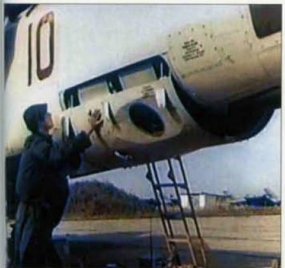
Centre and right: A technician loads a film cassette into one of the cameras as the pallet rests on the ground.
