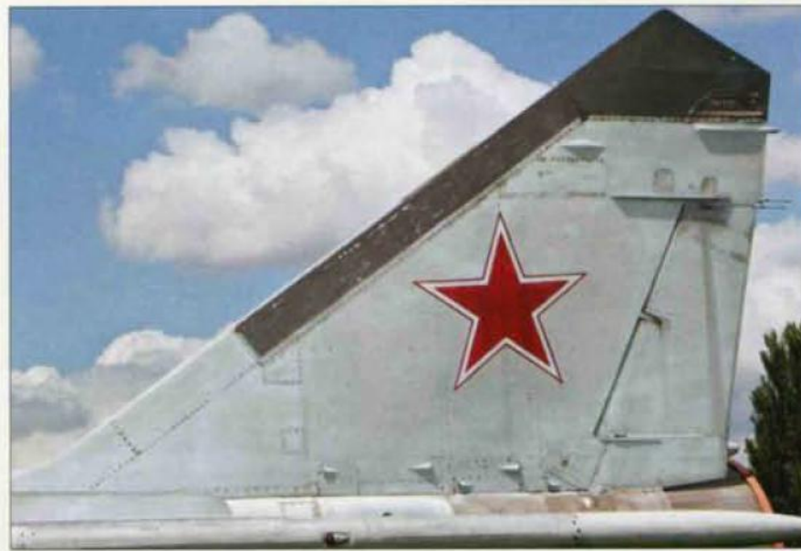
Above, left and right: The fins of the MiG-25 incorporate various navigation and communications antennae. The configuration of the dielectric portions on the port and starboard fins differs.
