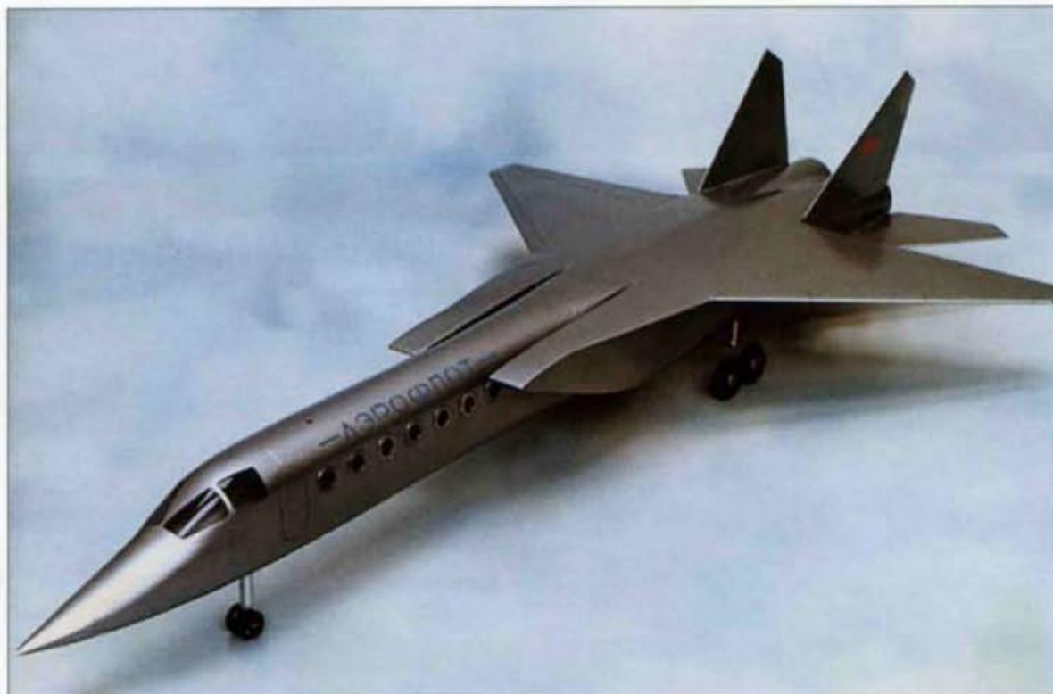
Above: A model of the proposed supersonic business jet derivative of the Ye-155 showing the all-new forward fuselage and main gear units. The number of cabin windows appears too large.
