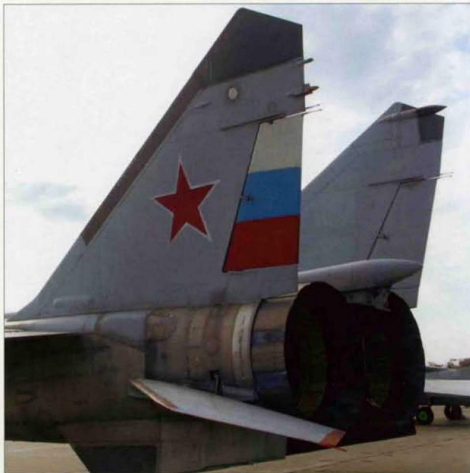
Left: The fins of the MiG-25 are canted slightly outward. Note the open brake parachute housing. Right: The tail unit of a MiG-25PD.
