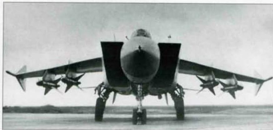
Below/bottom and below left/bottom left: Four more views of '05 Red' with a full load of dummy K-40R AAMs. Note that the air intake outer walls are canted outwards.
