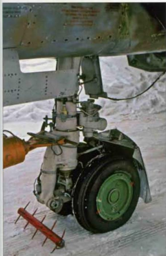
Above: Another view of a typical MiG-25's nose gear unit, showing the levered suspension and the steering mechanism/shimmy damper. Note the locally made 'hedgehog' strategically placed ahead of the nosewheels to puncture them in the event of unauthorised taxiing – a lesson learned from several hijackings of Soviet combat aircraft. Also of note are the red lines painted on the wheel rim and tyre to show instantly whether the tyre sits tight on the rim as it should.
