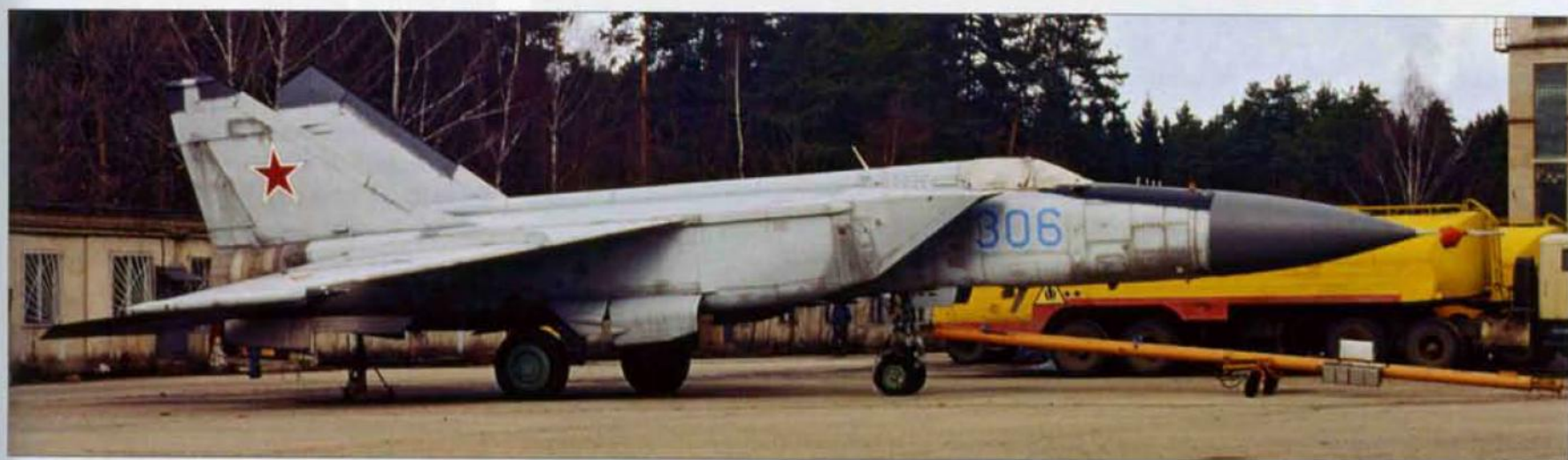
Top: At the end of its flying career the MiG-25PD prototype '306 Blue' was converted into the izdeliye 84-20 engine testbed. The longer nozzle of the AL-41F development engine is visible in the upper photo. The lower photo shows the machine languishing at the RSK MiG flight test facility in Zhukovskiy.
