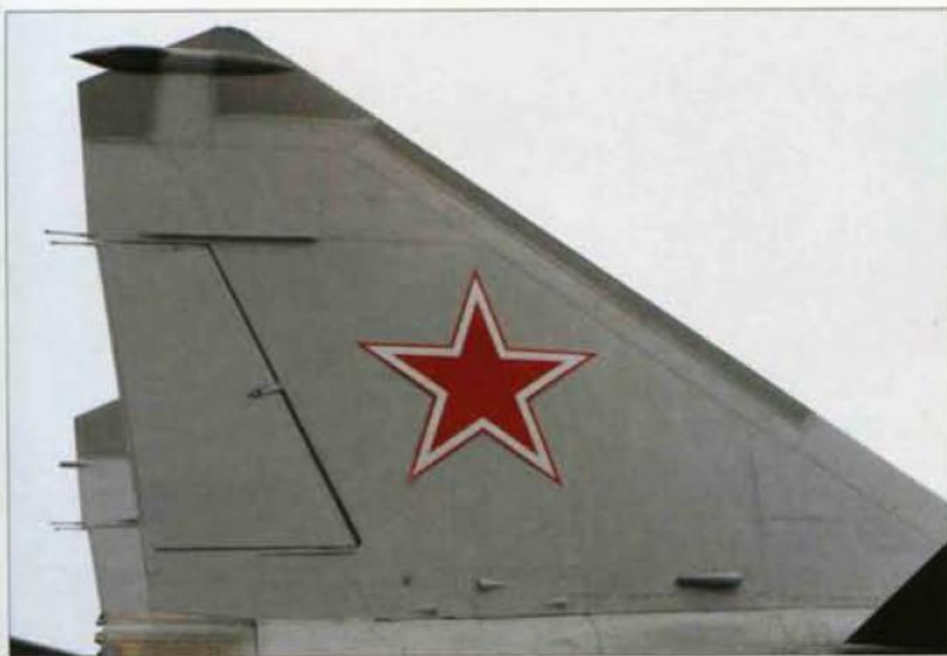
Above, left and right: The fins of the MiG-25 incorporate various navigation and communications antennae. The configuration of the dielectric portions on the port and starboard fins differs.
