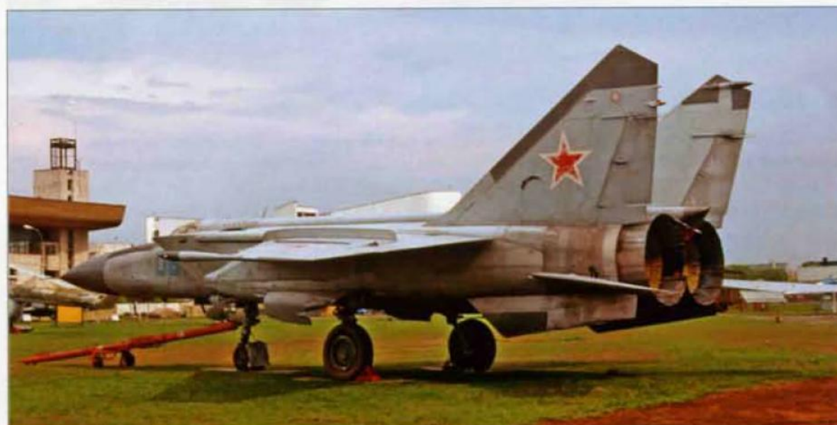
MiG-25PDS '08 Blue' (c/n N84018081) on display at the open-air museum at Moscow-Khodynka. This view shows the original short brake parachute housing that was retained after the PDS upgrade.
