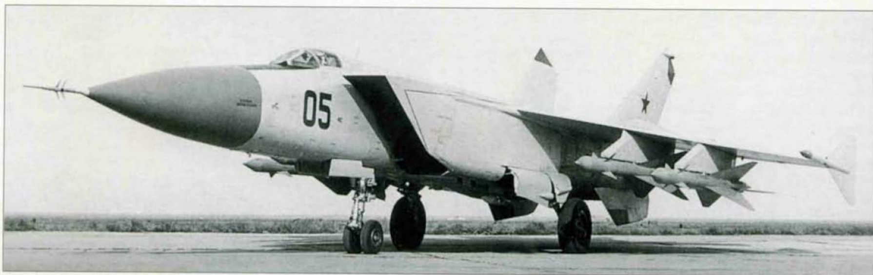
Above: '05 Red', the Ye-155P-5, after the addition of wingtip endplates. The air intakes' lower lips are fully deflected. Note the four wing pylons, the pale blue trim on the air intakes (which lack provisions for canards) and the 'Caution, fibreglass' stencil on the radome.
