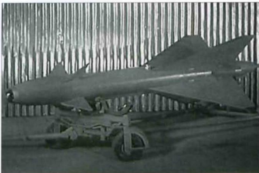
Left: A prototype K-40T medium-range IR-homing missile on a ground handling dolly.
