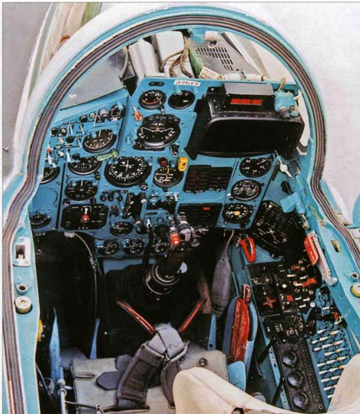
Above: The rear cockpit of the MiG-25PU-SOTN chase plane developed under the Buran space shuttle programme. Note the TV display on the right.
