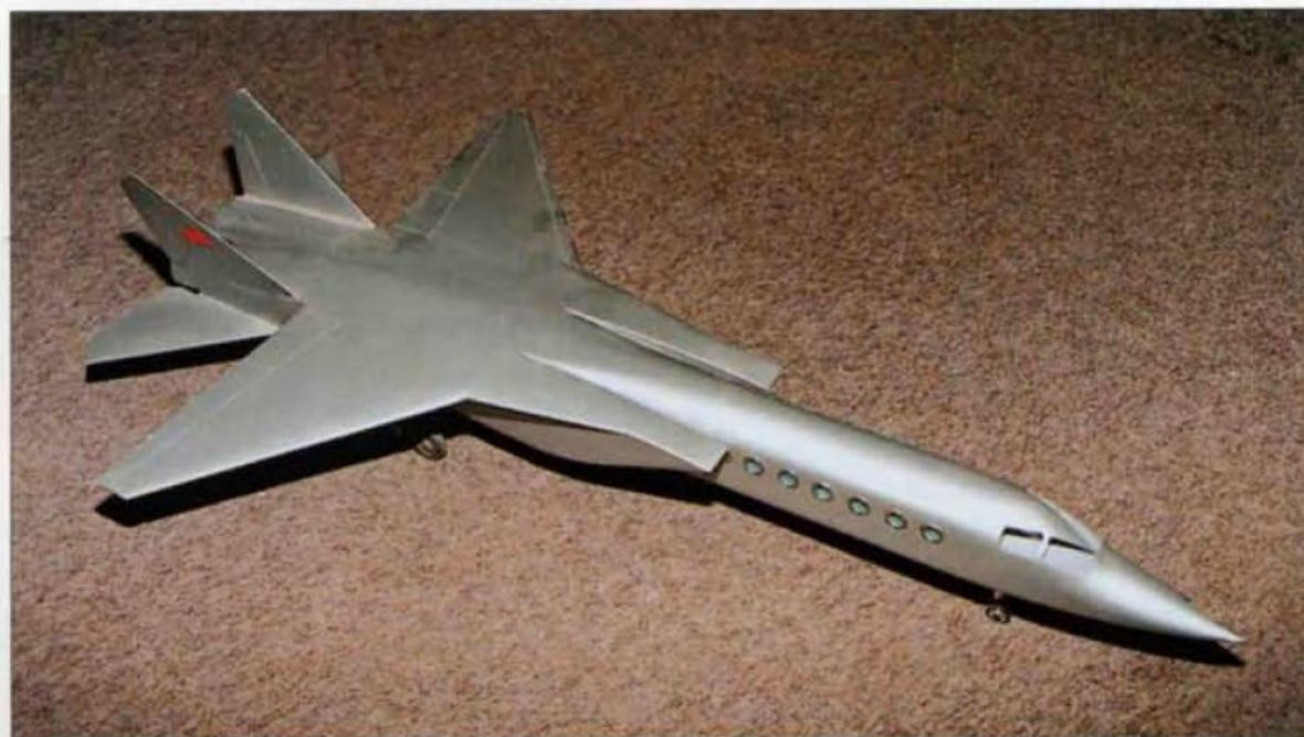
This view of the same model shows the modified wings of greater aspect ratio with LERXes and the large vertical tails.
