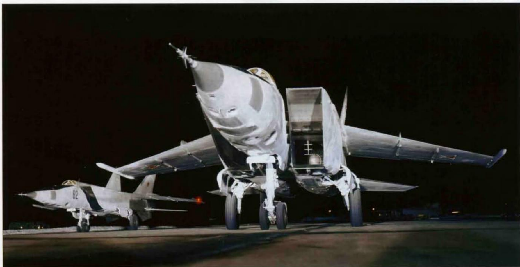
An atmospheric shot of two blue-coded MiG-25RBs taxiing out for a night sortie. Note the attachment fittings for the wing pylons.
