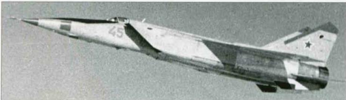
Top and above: A MiG-25R coded '45 Blue' shows the camera windows and the dielectric panels associated with SIGINT. The lack of wingtip anti-flutter weights shows this is a very early aircraft.
