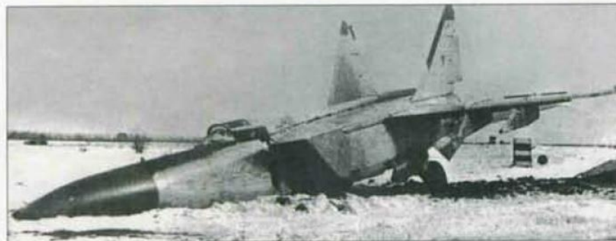
Left and above left: This MiG-25P coded '42 Blue' overran the runway when returning home from a practice sortie and was totalled, collapsing the nose and starboard main gear units and snapping the fuselage in the cockpit area. Note that the brake parachutes were not deployed.
