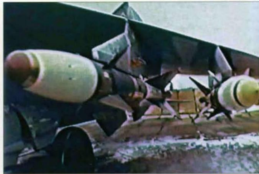
Right: A production R-40T (inboard) and a semi-active radar homing R-40R under the port wing of a MiG-25P.
