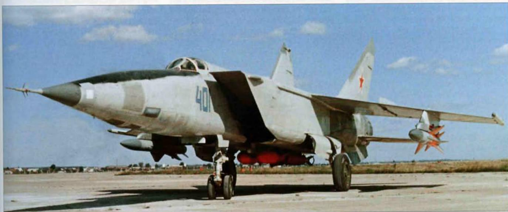
MiG-25RB '401 Blue' was one of several Foxbat-Bs modified under the MiG-25BM's development programme. The Kh-58U anti-radar missiles are well visible, as are the radar detection system antenna blisters low on the sides of the nose.
