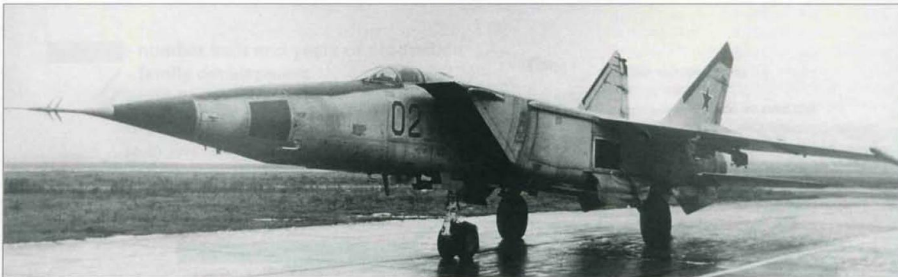
Above: MiG-25RBK '02 Blue' (c/n N02029210) served as an avionics testbed under the Buran space shuttle programme. Note the rectangular dielectric panel on the air intake trunk.
