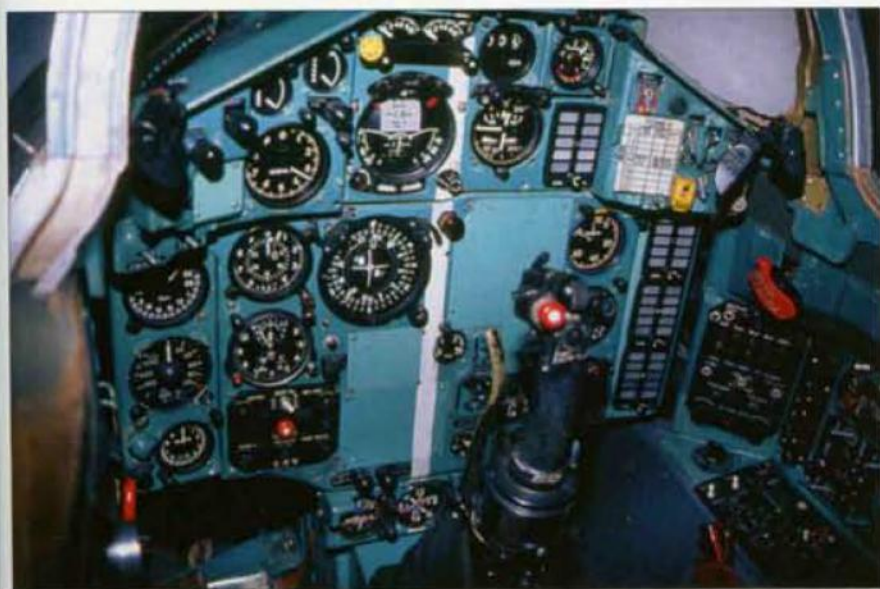
Two views of the cockpit of a MIG-25RB flight simulator. The lurid turquoise colour typical of Soviet aircraft is meant to reduce pilot fatigue.
