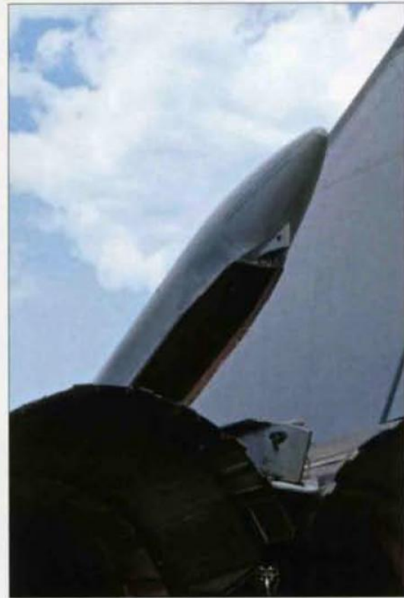
Top left: The original style of the brake parachute housing with a short pointed end.
