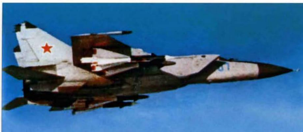
'07 Blue', an operational Soviet Air Force MiG-25P, toting a typical ordnance load – two IR-homing R-40Ts inboard and two semi-active radar homing R-40Rs outboard.
