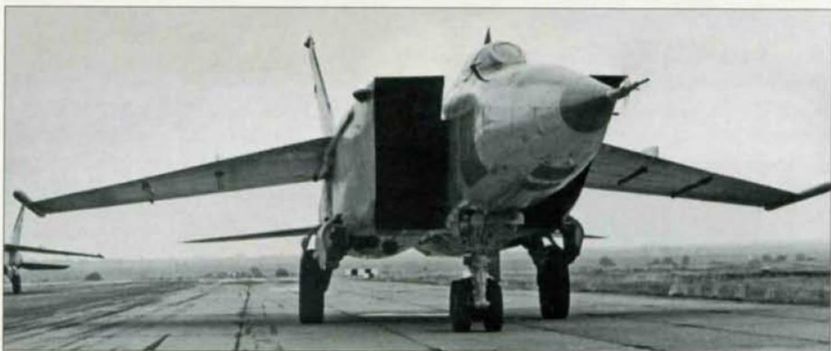
Above: Front view of a MiG-25RBS. Note the ECM blisters on the air intake trunks.
