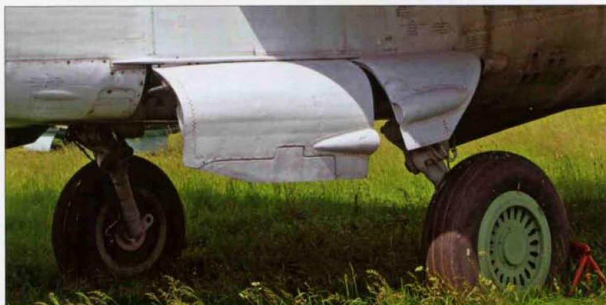
Above: Another view of a typical MiG-25's nose gear unit, showing the levered suspension and the steering mechanism/shimmy damper. Note the locally made 'hedgehog' strategically placed ahead of the nosewheels to puncture them in the event of unauthorised taxiing – a lesson learned from several hijackings of Soviet combat aircraft. Also of note are the red lines painted on the wheel rim and tyre to show instantly whether the tyre sits tight on the rim as it should.
