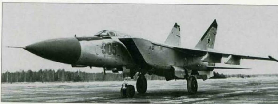
Above: '305 Blue', one of the MiG-25PD prototypes. The IRST fairing under the nose is clearly visible.
