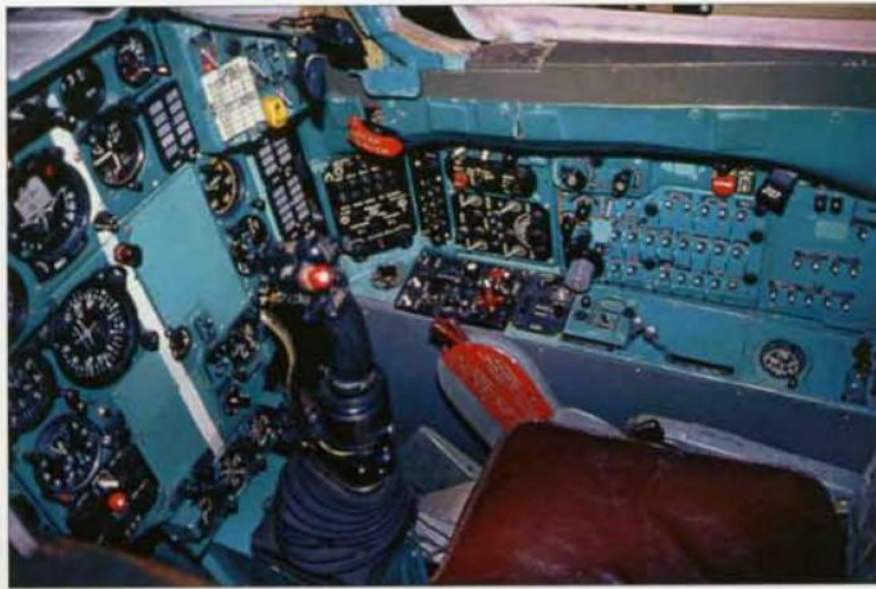
Two views of the cockpit of a MIG-25RB flight simulator. The lurid turquoise colour typical of Soviet aircraft is meant to reduce pilot fatigue.
