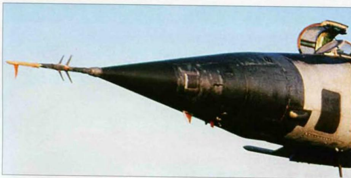
The nose of a MiG-25BM, showing the distinctive dielectric blisters and square-shaped dielectric panels of the radar detection suite.
