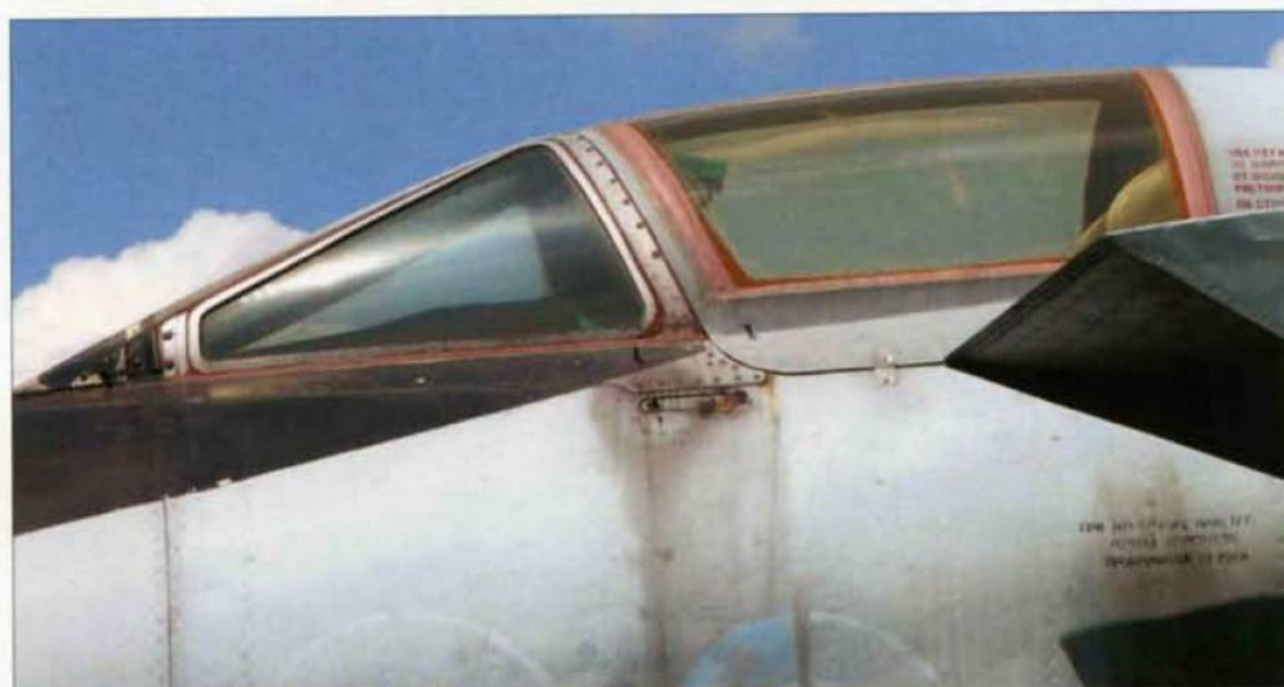
Above: The canopy of a MiG-25. Note the colour of the sealant around the edges of the transparencies.
