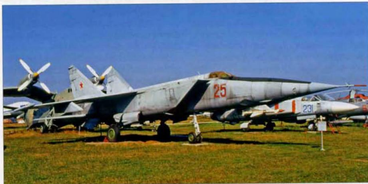
Refitted with production-style nose and tails, the Ye-155R-3 is now in the Central Russian Air Force Museum in Monino as '25 Red'. Note that MiG-25P missile pylons have been fitted in error.
