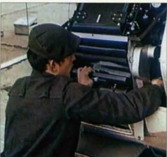
Centre and right: A technician loads a film cassette into one of the cameras as the pallet rests on the ground.
