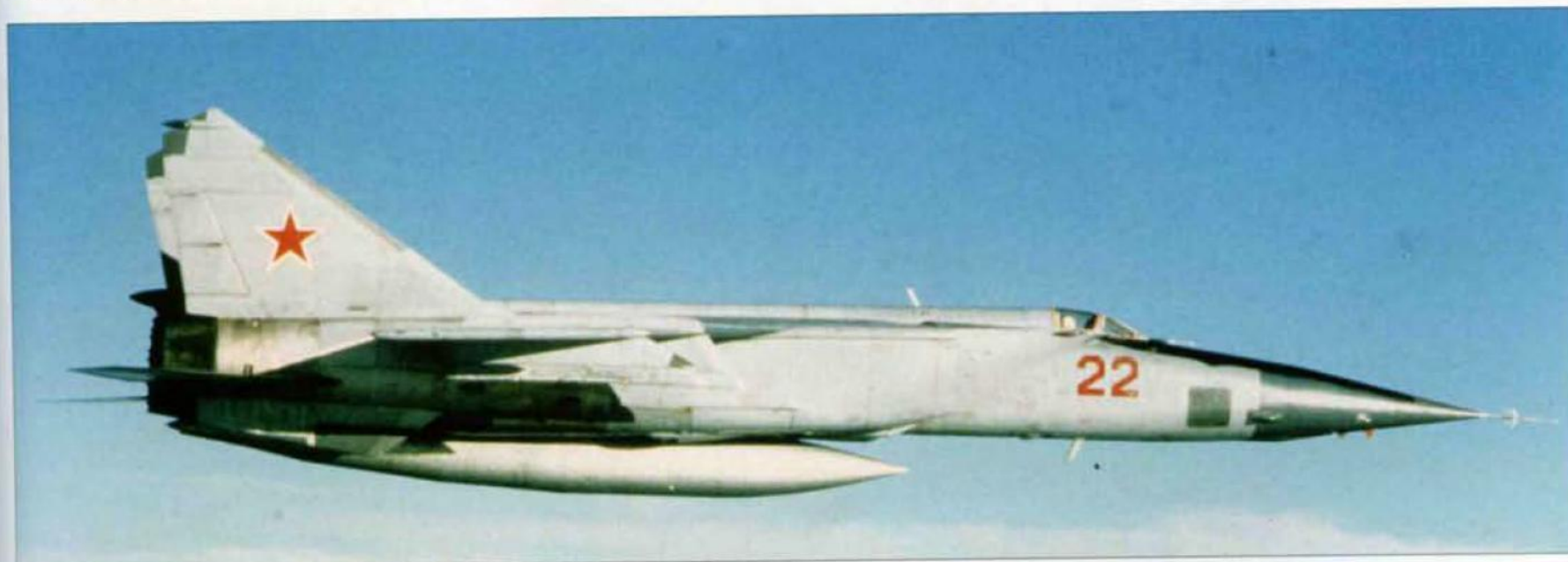
As this photo shows, the MiG-25BM was able to carry a drop tank. The SEAD version's colour scheme included a distinctive dark grey nose.
