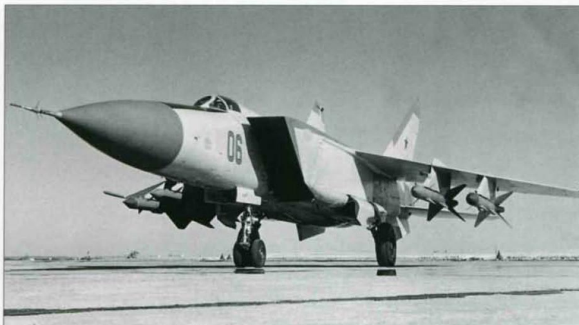
Left: '06 Blue', the Ye-155P-6 development aircraft, was the first MiG-25 to feature the production-standard large vertical tails.
