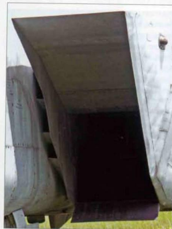
Top left: The port air intake of a MiG-25PD. Note the protective sheath on the lower intake lip preventing injuries to ground personnel.
