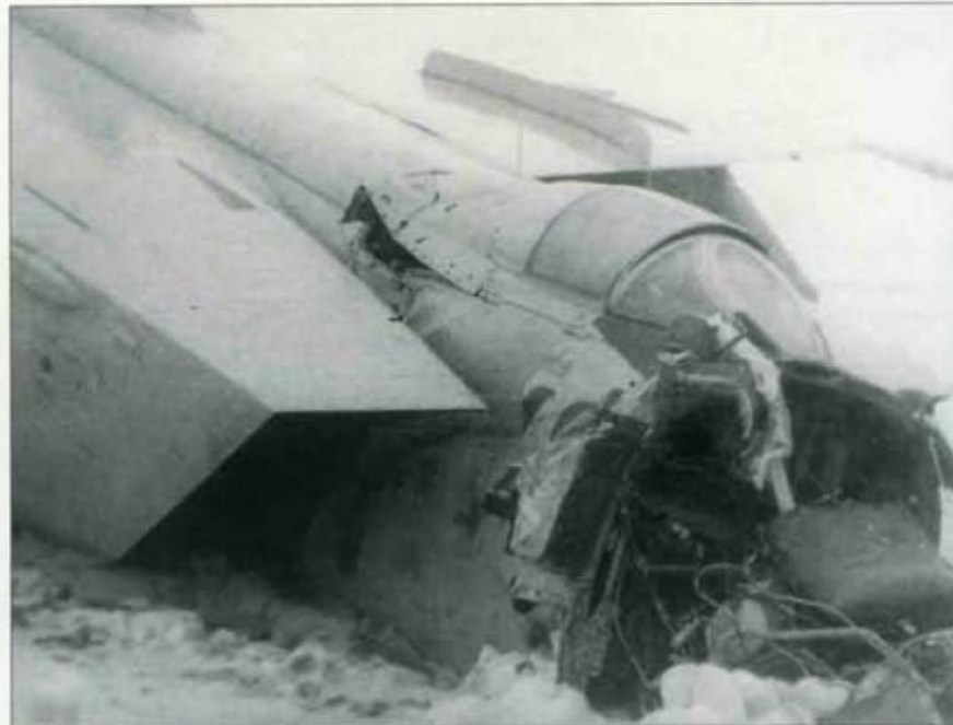
Left and above left: This MiG-25P coded '42 Blue' overran the runway when returning home from a practice sortie and was totalled, collapsing the nose and starboard main gear units and snapping the fuselage in the cockpit area. Note that the brake parachutes were not deployed.
