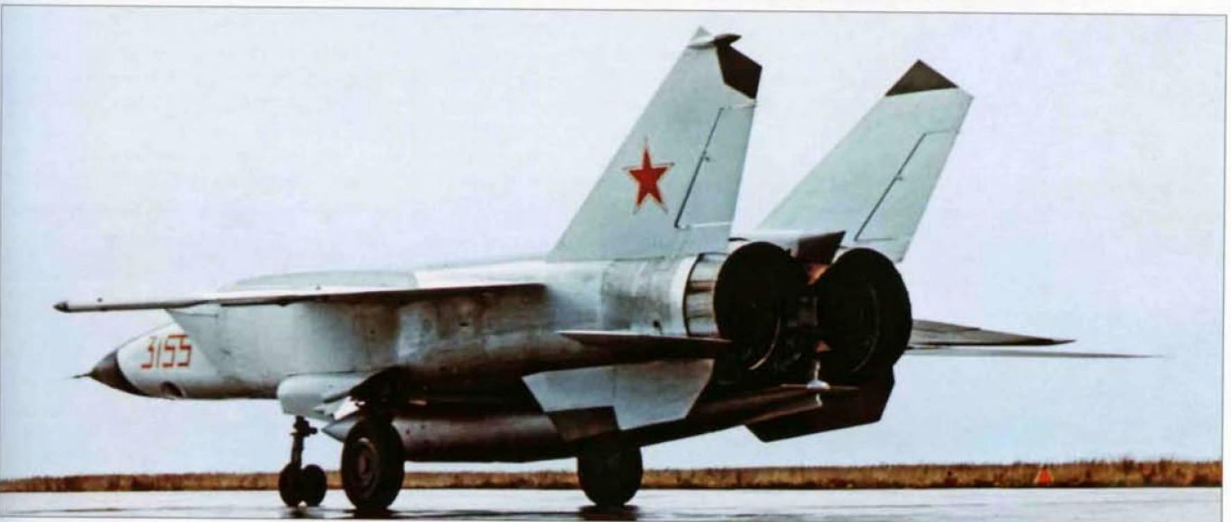
These three views of '3155 Red' illustrate well the redesigned fins with raked tips and the huge drop tank. Note also the difference in national insignia placement.
